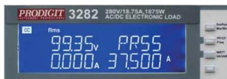
Turbo ON, Short 100mS 37.5A Test result
