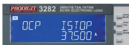
Turbo ON, OCP Istep 3.75 A Istop 37.5A Test result
