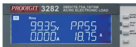
Turbo OFF, Short 100mS 18.75A Test result
